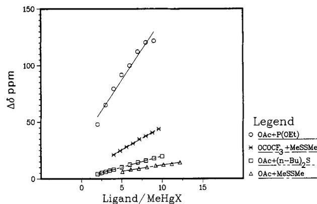
**Figure 3.** Plot of  $^{199}\text{Hg}$  chemical shifts vs. molar ratios of ligand/MeHgX.
