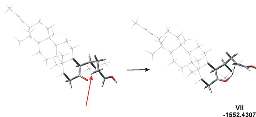
**Figure 4.** Formation of enol during structure optimization. The H atom from CH<sub>2</sub> (red arrow) of the protonated aldehyde moved to the C=O group, forming the rotamer VII (enol) stabilized by OH...CH= interaction (dotted line,  $d_{\text{OH}}$  1.022 Å,  $d_{\text{HC}}$  1.795 Å).
