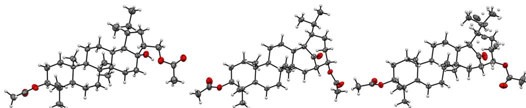
Figure 2. X-ray structure of 21 (left), 23 (middle), and 24 (right). Contour probability level: 50%.
