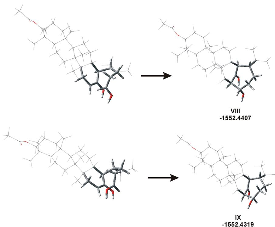
**Figure 5.** Transformation of 10 (enole form) to cyclic product 22. Depending on the orientation of the CH(=OH<sup>+</sup>) group, two configurations of the CH(OH) center have been obtained.
