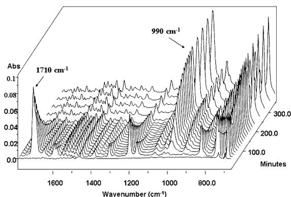
Figure 1. FTIR absorbance spectra during the addition of diethylzinc to benzaldehyde mediated by resin **7a**.
