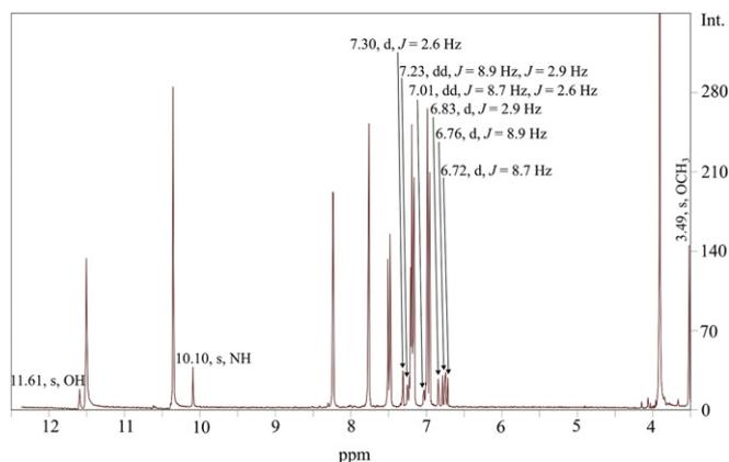
**Fig. 1.** <sup>1</sup>H NMR spectrum of compound **8i** in DMSO at ambient temperature. The relative integral intensity ratio of both conformers 1:0.15. For interpretation of signals of more intense conformer see [Experimental protocols](#).
