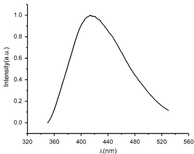
**Fig. 4** Solid-state emission spectrum of compound **1** ( $\lambda_{\text{ex}} = 270$  nm) at room temperature
