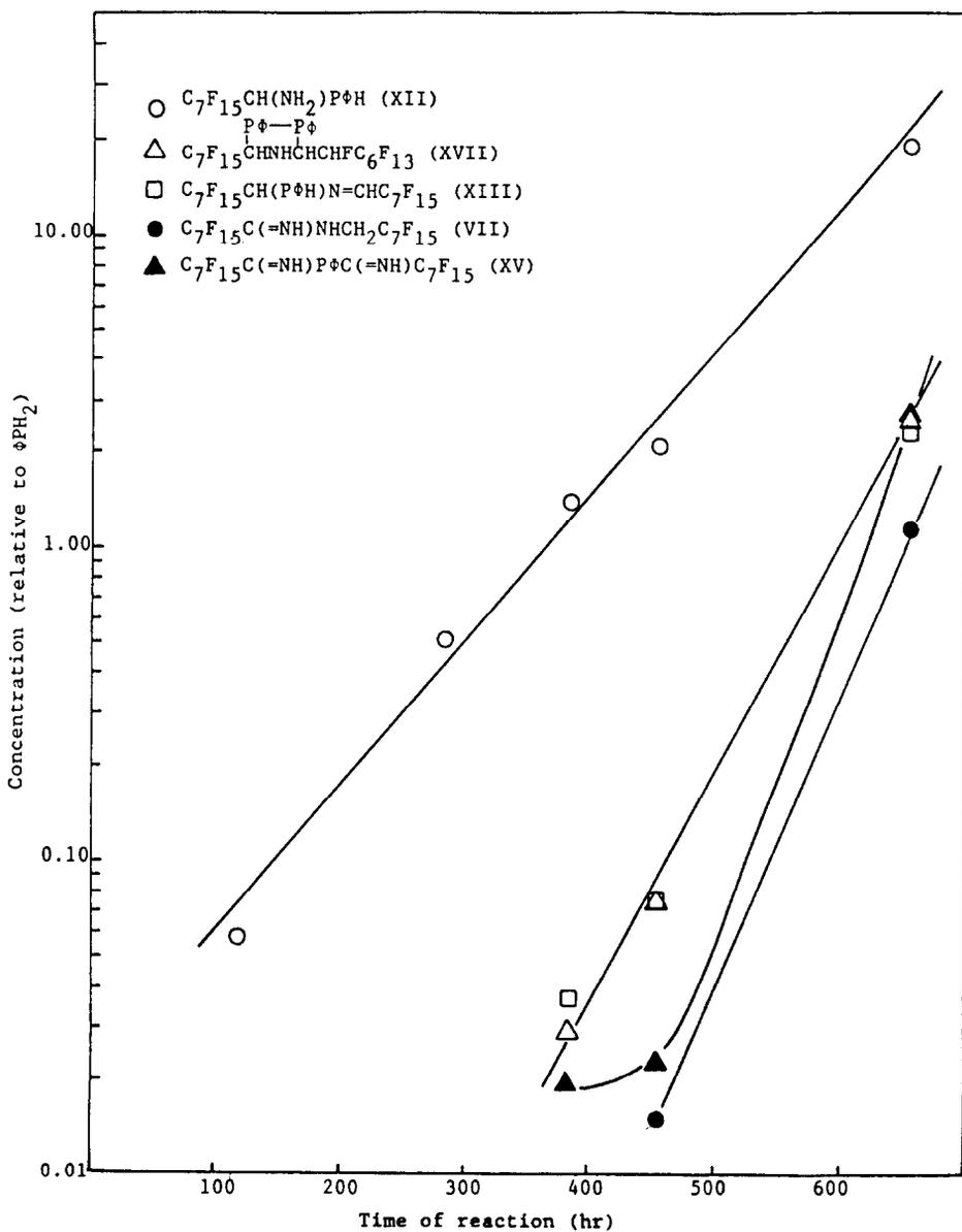
Fig. 4. Semi-log plot of concentration versus time for products from the reaction of phenylphosphine and perfluoro-n-octano-nitrile at 50°C in acetonitrile/Freon-113
