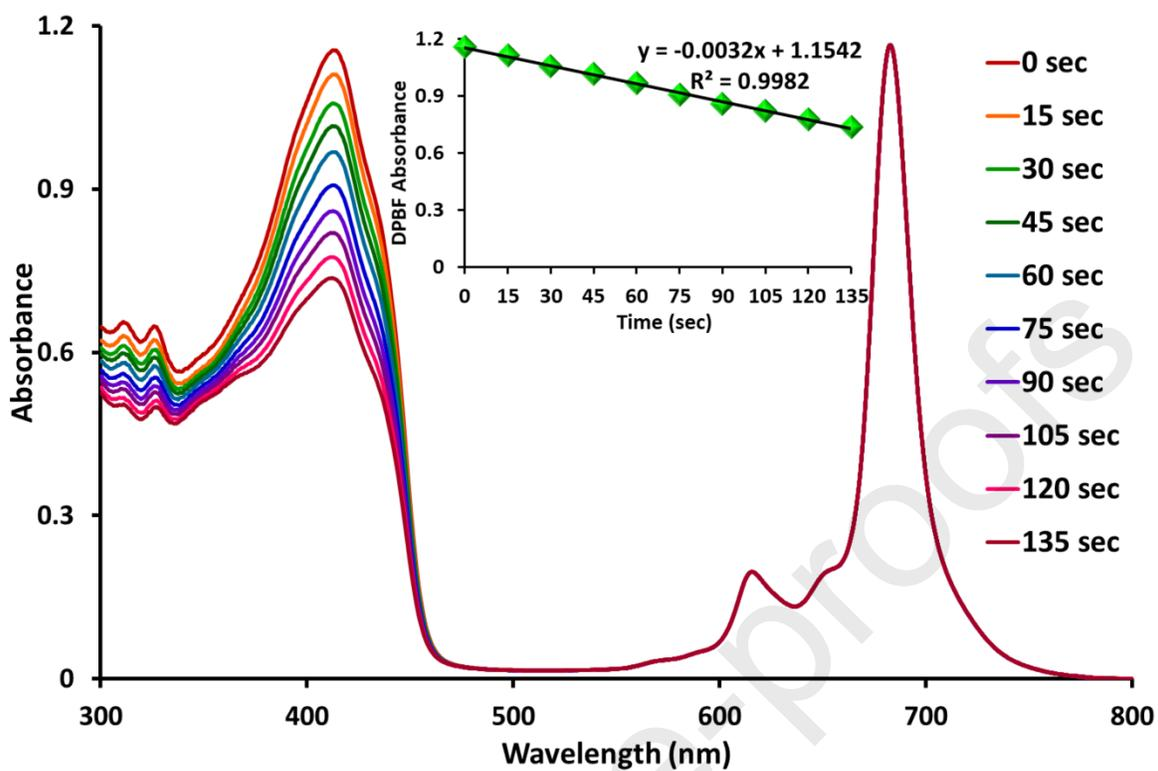
**Figure 7.** Absorption changes during the determination of singlet oxygen quantum yield for zinc(II) phthalocyanine (7) in DMF using DPBF as a singlet oxygen quencher.
