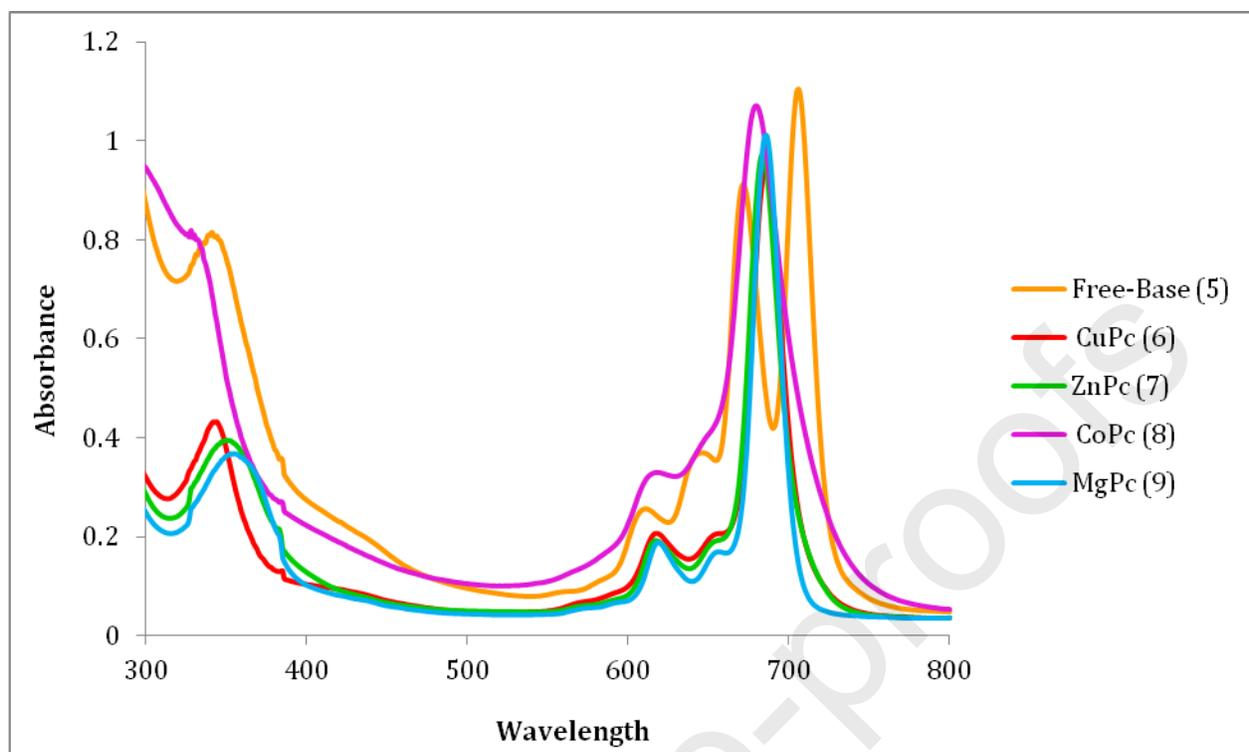
**Figure 4.** The ground state electronic absorption spectra of new free-base (5) copper(II) (6), zinc(II) (7), cobalt(II) (8) and magnesium(II) (9) phthalocyanines ( $C = 1.0 \times 10^{-5}$  M) in chloroform.
