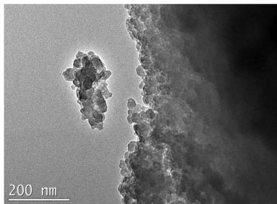
Fig. 3 The TEM of the aggregated silica nanoparticles loaded with the lipase.
