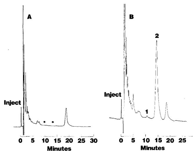
**Figure 1**—Chromatograms of outdated whole blood extract. Key: (A) unspiked sample (asterisks denote retention times of **1** and **2**, respectively); (B) spiked sample (11 ng/mL in whole blood). Conditions: column,  $\text{C}_{18}$  bonded silica ( $250 \times 4.0$  mm); mobile phase, 70% acetonitrile:0.005 M lauryl sulfate (pH 3.5); flow rate, 2.0 mL/min; detector, 254 nm at 0.01 AUFS (A) or 0.005 AUFS (B); column temperature, 40°C; sample volume, 20  $\mu\text{L}$ .
