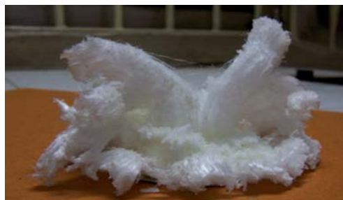
Fig. 1 Crystal growth of \text{AnHNO}_3 -I from the gel on filter paper after 8 h.
