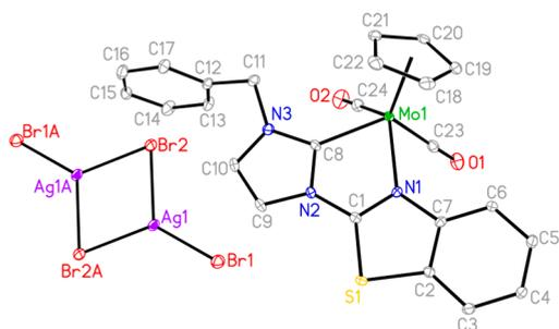
**Figure 5.** ORTEP diagram of one  $[\text{CpMo}(\text{CO})_2\text{NHC}]^+$  and  $[\text{Ag}_2\text{Br}_4]^{2-}$  of **8a** (30% probability ellipsoids). Hydrogen atoms are omitted. Selective bond lengths (Å) and angles (deg): Mo(1)–C(24) 1.966(6); Mo(1)–C(23) 1.991(6); Mo(1)–C(8) 2.143(5); Mo(1)–N(1) 2.195(5); C(24)–Mo(1)–C(23) 75.8(3); C(8)–Mo(1)–N(1) 72.3(2).
