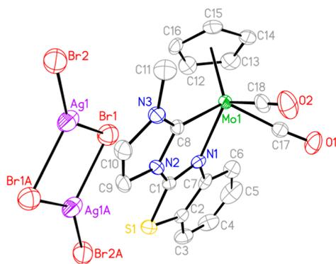
**Figure 4.** ORTEP diagram of one  $[\text{CpMo}(\text{CO})_2\text{NHC}]^+$  and  $[\text{Ag}_2\text{Br}_4]^{2-}$  of **7a** (30% probability ellipsoids). Hydrogen atoms are omitted. Selective bond lengths (Å) and angles (deg): Mo(1)–C(18) 1.95(1); Mo(1)–C(17) 1.98(1); Mo(1)–C(8) 2.161(9); Mo(1)–N(1) 2.206(8); C(18)–Mo(1)–C(17) 75.0(5); C(8)–Mo(1)–N(1) 72.0(3).
