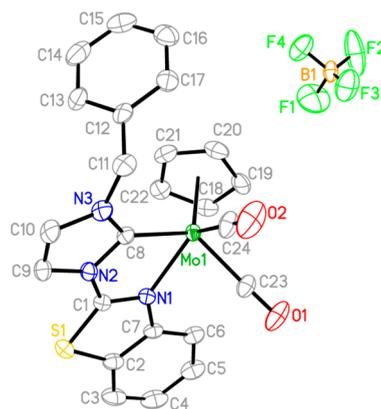
**Figure 7.** ORTEP diagram of **8b** (30% probability ellipsoids). Hydrogen atoms are omitted. Selective bond lengths (Å) and angles (deg): Mo(1)–C(23) 1.988(4); Mo(1)–C(24) 1.944(3); Mo(1)–C(8) 2.162(3); Mo(1)–N(1) 2.206(2); C(18)–Mo(1)–C(19) 75.2(2); C(8)–Mo(1)–N(1) 72.6(1).
