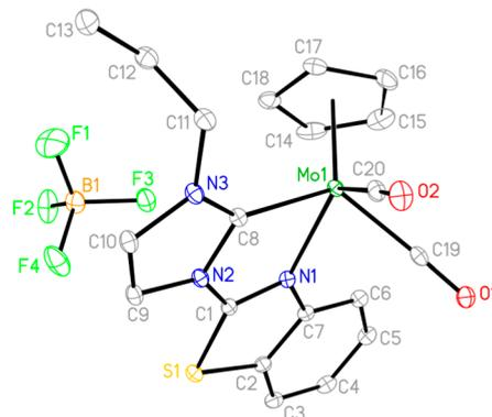
**Figure 8.** ORTEP diagram of **9b** (30% probability ellipsoids). Hydrogen atoms are omitted. Selective bond lengths (Å) and angles (deg): Mo(1)–C(20) 1.975(2); Mo(1)–C(19) 1.994(2); Mo(1)–C(8) 2.143(2); Mo(1)–N(1) 2.196(1); C(20)–Mo(1)–C(19) 75.45(7); C(8)–Mo(1)–N(1) 72.58(6).
