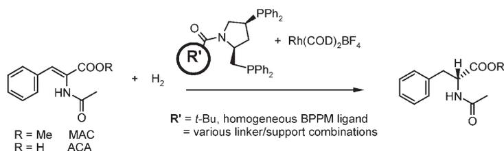
**Figure 2.** Test reaction using various rhodium-4-(diphenylphosphino)-2-(diphenylphosphinomethyl)-pyrrolidine (Rh-PPM) catalysts.
