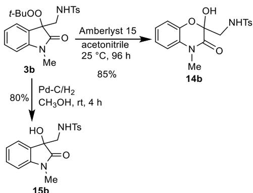
could be removed by hydrogenation in methanol at rt to afford **15b** with high yield.
