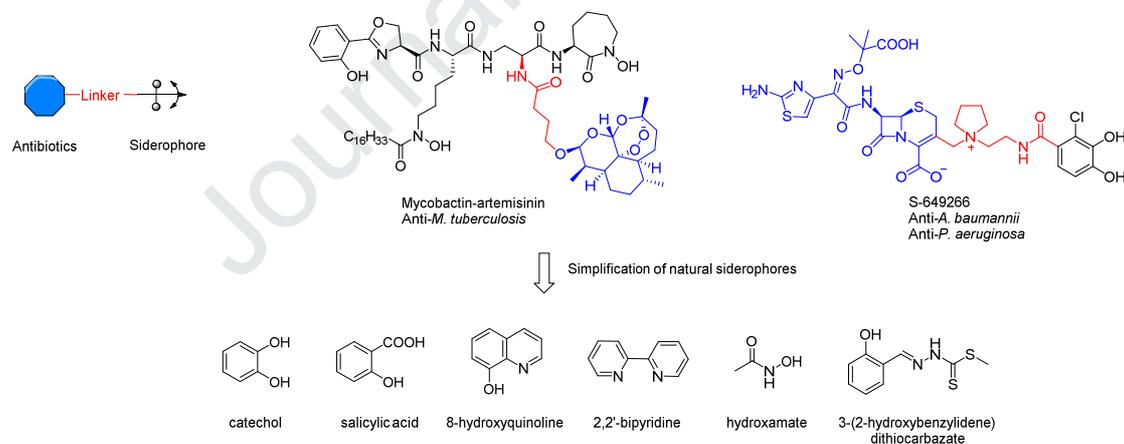
**Figure 1.** Generalized structure of a siderophore mediated drug delivery system and two successful examples of siderophore conjugation: the mycobactin-artemisinin conjugate and the single bidentate catechol-cephalosporin conjugate S-649266 [27,28].
