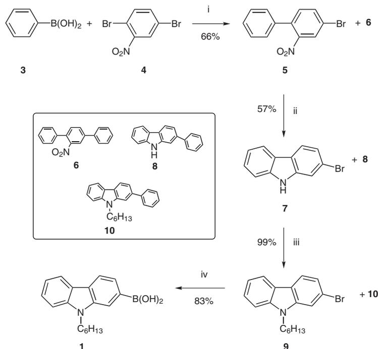
**Scheme 1** Reagents and conditions: (i) Pd(PPh<sub>3</sub>)<sub>4</sub> (3% equiv), aq 2 M Na<sub>2</sub>CO<sub>3</sub> (3 equiv), toluene, 90 °C, 5.5 h; (ii) (EtO)<sub>3</sub>P, reflux, 10 h; (iii) *t*-BuOK (1.2 equiv), DMF, 20 °C, 2 h; 1-bromohexane (1.5 equiv), 130 °C, 65 h; (iv) *n*-BuLi (1.2 equiv), THF, –78 °C, 2 h; (*i*-PrO)<sub>3</sub>B (3.0 equiv), –78 to 20 °C, 16 h; concd HCl, 20 °C, 2 h.
