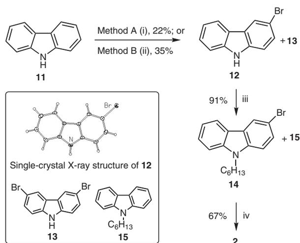
**Scheme 2** Reagents and conditions: (i) *n*-BuLi (1.0 equiv), –78 °C, 15 min; Me<sub>3</sub>SiCl (1.0 equiv), 20 °C, 3 h; Br<sub>2</sub> (1.0 equiv), –78 °C, 1 h; 20 °C, 2 h (ii) Br<sub>2</sub> (1.1 equiv), DMF, 0–20 °C, 1–27 h; (iii) *t*-BuOK (1.2 equiv), DMF, 20 °C, 1 h; 1-bromohexane (1.5 equiv) 130 °C, 65 h; (iv) *n*-BuLi (1.2 equiv), THF, –78 °C, 1 h; (*i*-PrO)<sub>3</sub>B (3.0 equiv), –78 to 20 °C, 22 h; concd HCl (5.0 equiv), 20 °C, 2 h.
