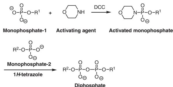
**Scheme 1.** Formation of diphosphate compounds by the cross-coupling reaction of two monophosphate.
