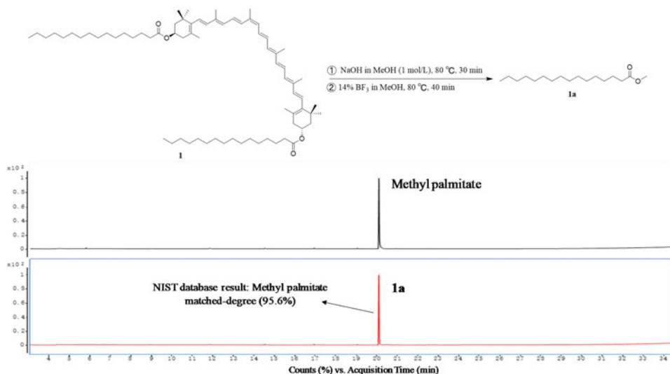
**Figure 2.** The product (**1a**) prepared from **1** and methyl palmitate were compared by GC-MS.
