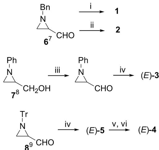
**Scheme 2.** Reagents and conditions: (i) (EtO)<sub>2</sub>P(O)CH<sub>2</sub>CN, NaH, THF, 0 °C; (ii) (EtO)<sub>2</sub>P(O)CH<sub>2</sub>CO<sub>2</sub>Et, NaH, THF, 0 °C; (iii) oxalyl chloride, DMSO, CH<sub>2</sub>Cl<sub>2</sub>, -78 °C; (iv) (EtO)<sub>2</sub>P(O)CH<sub>2</sub>CO<sub>2</sub>Et, NaH, CH<sub>2</sub>Cl<sub>2</sub>, 0 °C; (v) TFA, MeOH, CHCl<sub>3</sub>; (vi) (PhCO)<sub>2</sub>O, NEt<sub>3</sub>, CHCl<sub>3</sub>.
