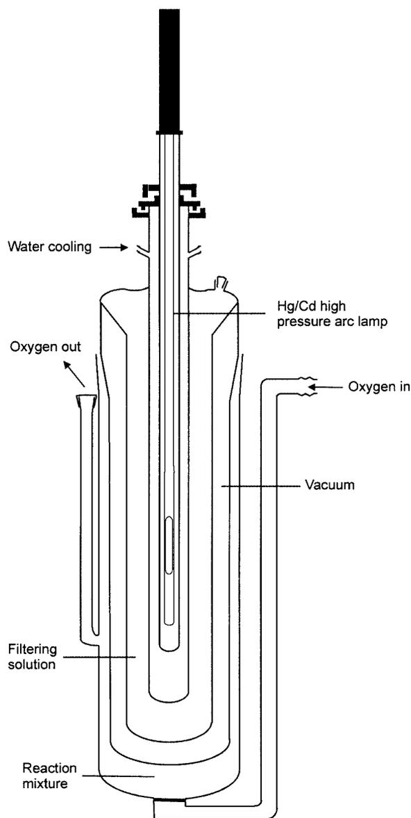
Figure 4. Photoreactor for the synthesis of dioxirane **2b**
