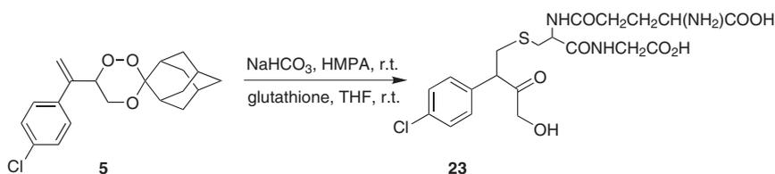
**Scheme 5** Synthesis of a 3-aryl-1-hydroxy-4-sulfanylbutan-2-one amino acid derivative from a trioxane and glutathione**Table 2** Conditions and Yields of Conjugate Additions of Amines and Thiols to 3-Aryl-1-hydroxybut-3-en-2-ones<sup>a</sup>
