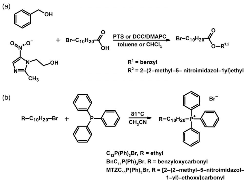
**Scheme 1** Synthesis of amphiphilic phosphonium salts: (a) preparation of esters, (b) quaternisation of triphenylphosphine with bromoalkanes
