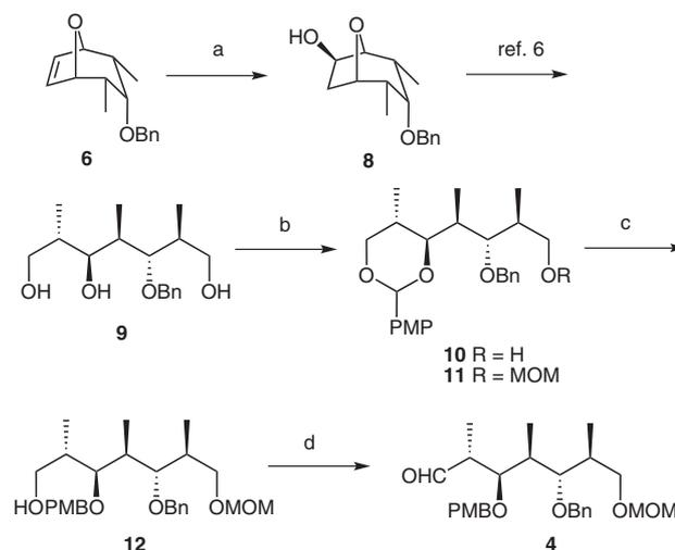
**Scheme 2** Reagents and conditions: (a) (+)-IPC<sub>2</sub>BOMe, THF, –20 °C, 5 d, 92%; (b) (i) 1-(MeO)<sub>2</sub>CH-4-MeOC<sub>6</sub>H<sub>3</sub>, anhyd CH<sub>2</sub>Cl<sub>2</sub>, CSA, 0 °C to r.t., 2 h, 85%; (ii) MOM-Cl, DIPEA, anhyd CH<sub>2</sub>Cl<sub>2</sub>, 0 °C, 3 h, 75%; (c) DIBAL-H, anhyd CH<sub>2</sub>Cl<sub>2</sub>, 0 °C, 1 h, 80%; (d) IBX, anhyd DMSO, anhyd CH<sub>2</sub>Cl<sub>2</sub>, 0 °C, 2 h, 90%.
