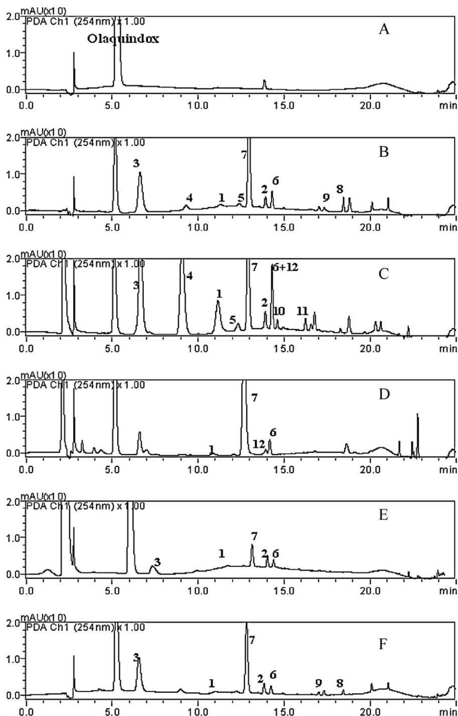
**Fig. 1.** LC–UV chromatograms of olaquinox standard solution (A), and the stressed olaquinox by H<sub>2</sub>O for 12 h (B); 0.1 N HCl for 12 h (C); 0.1 N NaOH for 24 h (D); 30% H<sub>2</sub>O<sub>2</sub> for 12 h (E); as well as UV fluorescent light at room temperature for 12 h (F).
