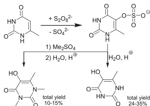
**Scheme 1.** Synthesis of 5-hydroxy-6-methyluracil and 5-hydroxy-1,3,6-trimethyluracil.
