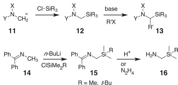
Fig. 3. Alpha-amino silane synthesis by metalation–alkylation.
