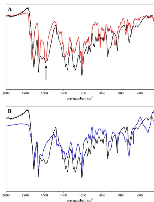
**Figure 4.** IR spectra of DHA and HA. (A) DHA (red) versus crude HA (black); and (B) Extensively washed HA (blue) versus crude HA (black). Spectra measured with a diamond cell ATR and show the common strong carboxyl band at 1587  $\text{cm}^{-1}$  (black arrow) which is present in DHA and crude HA. The band 1584  $\text{cm}^{-1}$  is absent in purified HA.
