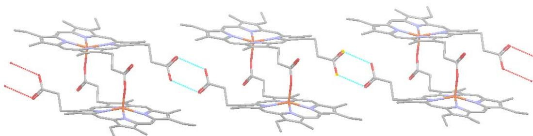
**Figure 1** Propionic acid structural roles in HZ and HA,  $[\text{Fe}(\text{protoporphyrinato})]_2$ . Each heme has one Fe-O bond to one propionate and the second propionic acid forms a H-bonded dimer. H-bonds are shown as blue or red dashed lines with a conventional CPK atomic coloring scheme employed. Structure shown taken from the CDC entry XETXUP and shows only one set of positions for the disordered vinyl groups.<sup>13</sup>
