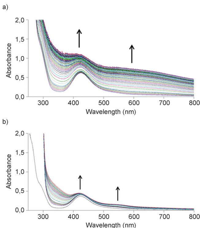
**Figure 2.** Time-dependent UV/Vis spectra (up to 24 h) of compound **1**  $10^{-3}$  M dissolved in  $20 \text{ mmol L}^{-1}$  ammonium acetate buffer, pH 6.8 (a), and in the presence of HEWL (b).  $[\text{compound } \mathbf{1}] = 5 \times 10^{-4} \text{ mmol L}^{-1}$ , complex/protein = 1:1.
