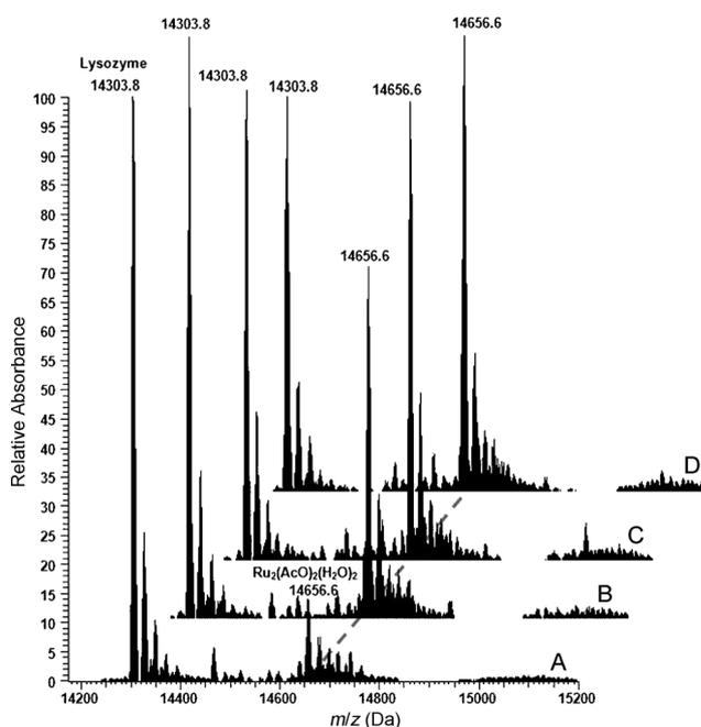
**Figure 3.** Deconvoluted ESI-MS of HEWL treated with  $10^{-3} \text{ mol L}^{-1}$   $[\text{Ru}_2(\mu\text{-O}_2\text{CCH}_3)_4\text{Cl}]$  (complex/protein = 10:1) in  $20 \text{ mmol L}^{-1}$  ammonium acetate buffer, pH 6.8 recorded after 6 h (A), 24 h (B), 48 h (C), and 72 h (D) of incubation at RT.
