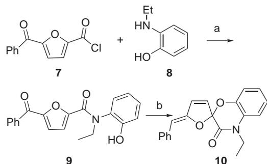
**Scheme 3** Synthesis of lactam **10**. *Reagents and conditions:* (a)  $\text{Et}_3\text{N}$ ,  $\text{CH}_2\text{Cl}_2$ , 89%; (b) i.  $\text{NaBH}_4$ , MeOH; ii. CSA,  $\text{CH}_2\text{Cl}_2$ , r.t., 5 h, 84%
