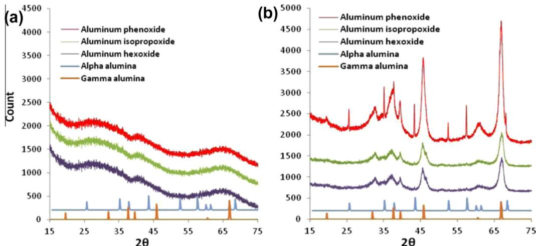
Fig. 7. X-ray diffraction patterns of (a) APh, AH, and AIP calcined at 550 °C (b) APh, AH, and AIP calcined at 1000 °C.
