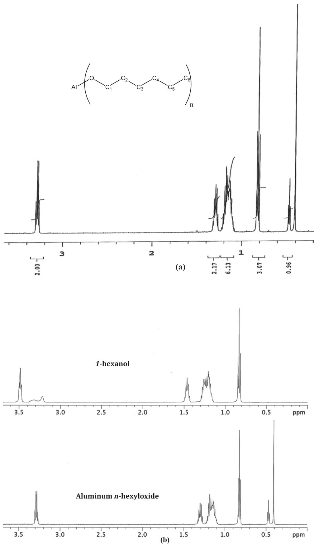
Fig. 1. (a)  $^1\text{H}$  NMR of aluminum *n*-hexyloxide, and (b)  $^1\text{H}$  NMR of aluminum *n*-hexyloxide and 1-hexanol comparison.
