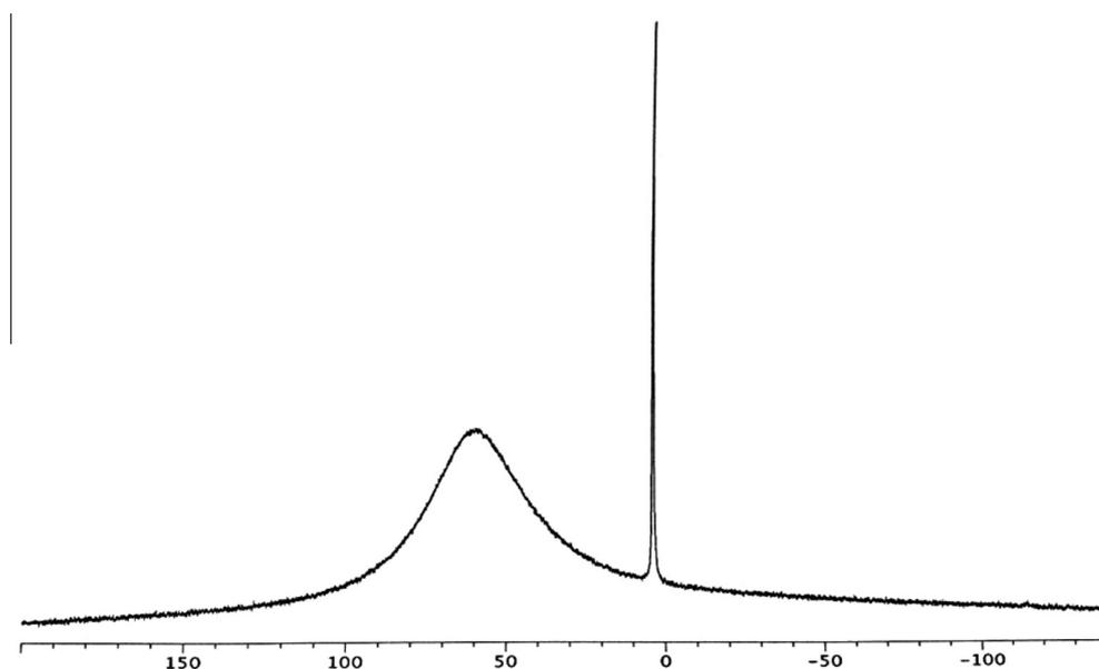
Fig. 5.  $^{27}\text{Al}$  NMR of aged aluminum isopropoxide.
