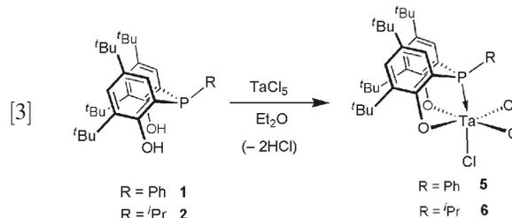
The synthesis of **5** and **6** is strongly linked to the concentration of the reagents in the reaction mixture. For example, reaction of **1** with  $\text{TaCl}_5$  in highly concentrated solution
