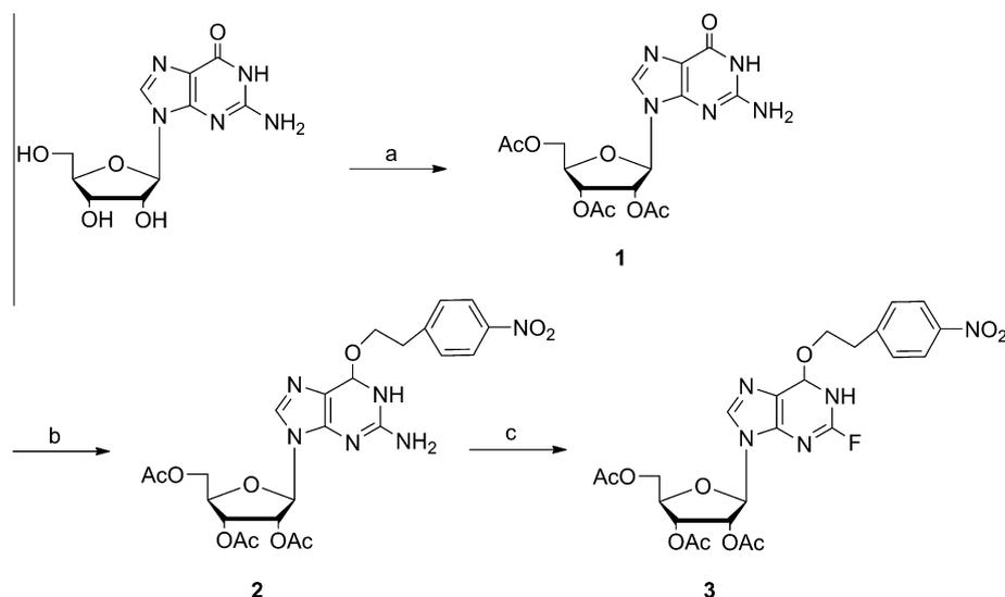
**Scheme 1.** Preparation of  $N^2$ -fluoro-2',3',5'- $O$ -triacetyl- $O^6$ -[2-(4-nitrophenyl)ethyl]inosine; (a) acetic anhydride, DMAP,  $\text{Et}_3\text{N}$ ,  $\text{AcCN}$ ,  $4^\circ\text{C}$  to rt; (b) NPE,  $\text{PPh}_3$ , DIAD, toluene, rt; (c) HF/pyridine,  $t\text{BuONO}$ , pyridine,  $-40^\circ\text{C}$ .
