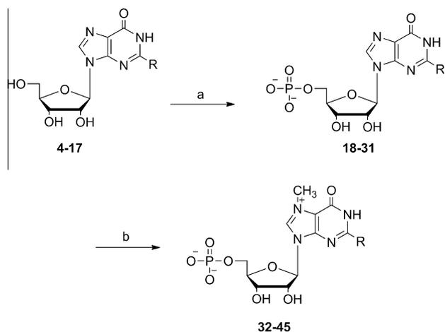
**Scheme 3.** Preparation of  $N^2$ -modified mononucleotide cap analogues (a) POCl<sub>3</sub>, trimethyl phosphate, 4 °C; (b) methyl iodide, DMSO, rt. <sup>a</sup>R corresponds to various substituents at the N<sub>2</sub> position of guanosine (see Scheme 2, numbers in brackets).
