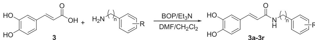
Fig. 3. Synthesis of compounds 3a–3r using BOP as a condensing reagent.
