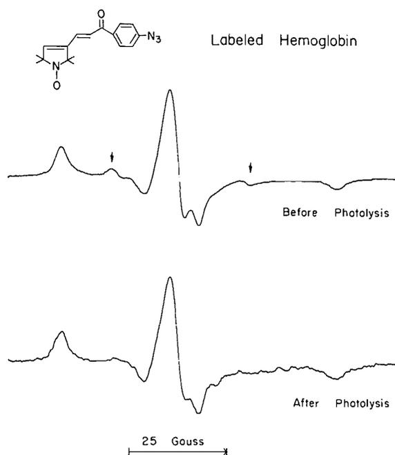
FIG. 1. The 25°C esr spectra of hemoglobin covalently labeled with nitroxide **21** before and after photolysis. The arrows in the top spectrum indicate the mobile component, the relative amount of which is reduced when the preparation is exposed to visible light.
