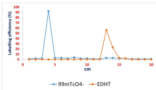
Fig. 2. Radiochromatogram of  $^{99m}\text{Tc}$ -EDHT using ITLC-SG in Ethanol, Ammonia and Water (2:1:5 v/v) at room temperature (25 °C).
