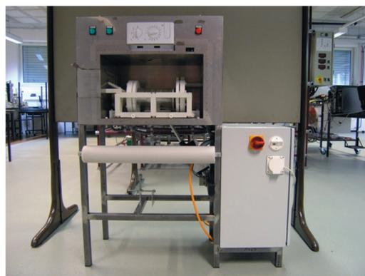
Fig. 6 The microwave barrel reactor with controller box.
