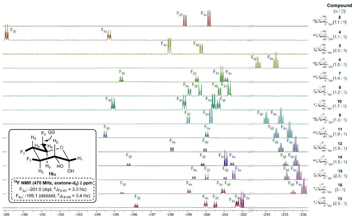
**Figure 2.** Direct comparison of <sup>19</sup>F resonances of fluorinated glucose analogues **3–16** (<sup>19</sup>F NMR (470 MHz, acetone-*d*<sub>6</sub>)) and proposed conformation of 3,4,6-trifluoroglucose **16α** showing the GG conformation of F-6 and long-range (<sup>4</sup>*J*) couplings in bold.
