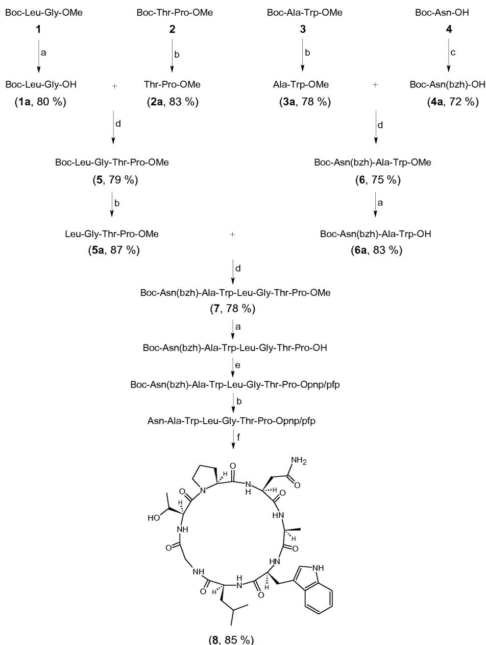
Scheme 1. Synthetic route to the cycloheptapeptide (annomuricin B) **8**. Reaction conditions: a = LiOH·H<sub>2</sub>O (1 : 1), r. t., 1 h; b = TFA, CHCl<sub>3</sub>, r. t., 1 h; c = benzhydrol, GAA, H<sub>2</sub>SO<sub>4</sub>, r. t., 30 min; d = EDC·HCl or DIPC, TEA or NMM, THF or DMF, r. t., 24–36 h; e = DIPC, pnp/pfp, r. t., 12 h; f = TEA or NMM or pyridine, 7 d, 0 °C.
