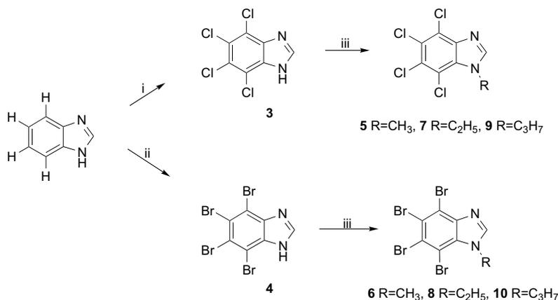
**Scheme 2.** Reagents and conditions: (i) HCl, HNO<sub>3</sub>, reflux; (ii) HNO<sub>3</sub>, Br<sub>2</sub>, reflux; (iii) CH<sub>3</sub>I (or C<sub>2</sub>H<sub>5</sub>I or C<sub>3</sub>H<sub>7</sub>I), CH<sub>3</sub>CN, DBU.
