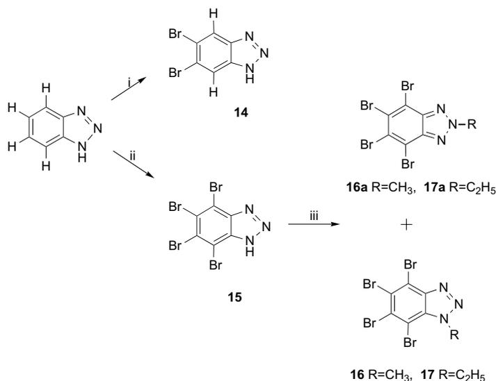
**Scheme 3.** Reagents and conditions: (i) H<sub>2</sub>SO<sub>4</sub>, Ag<sub>2</sub>SO<sub>4</sub>, Br<sub>2</sub>, room temperature; (ii) HNO<sub>3</sub>, Br<sub>2</sub>, reflux; (iii) CH<sub>3</sub>I (or C<sub>2</sub>H<sub>5</sub>I), CH<sub>3</sub>CN, DBU.
