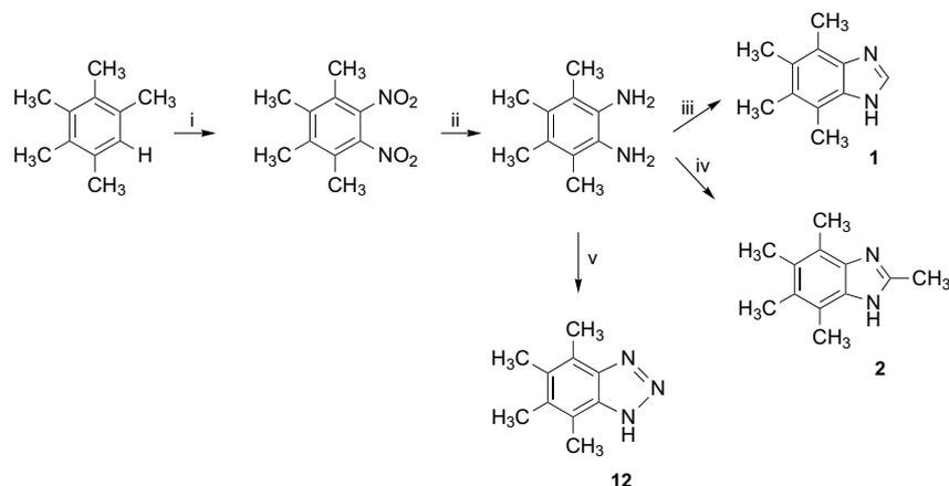
**Scheme 1.** Reagents and conditions: (i) fuming HNO<sub>3</sub>, concentrated H<sub>2</sub>SO<sub>4</sub>, <10 °C; (ii) SnCl<sub>2</sub>, HCl, reflux; (iii) HCOOH; (iv) CH<sub>3</sub>COOH; (v) NaNO<sub>2</sub>, HCl.
