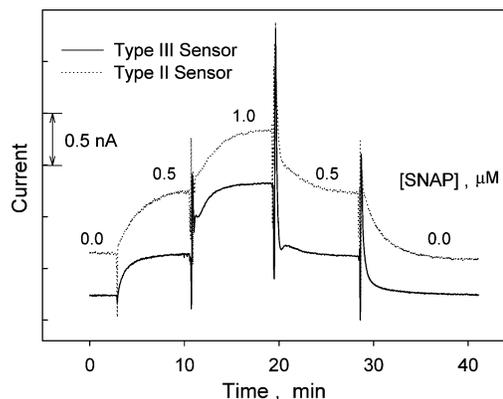
**Figure 5.** Dynamic recordings illustrating real-time reversibility of type II and type III RSNO sensors in amperometric response to varying concentrations of SNAP.
