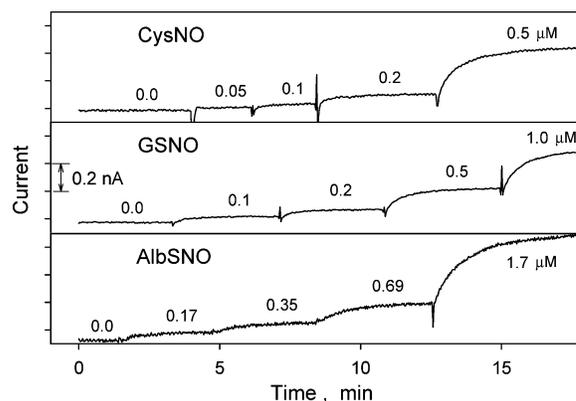
**Figure 3.** Typical real-time current recordings for type III sensor in response to low levels of three endogenous RSNO species. Sample solutions contain 10  $\mu\text{M}$  EDTA and 10  $\mu\text{M}$  ascorbate as a reducing agent, along with varying RSNO concentrations at room temperature.
