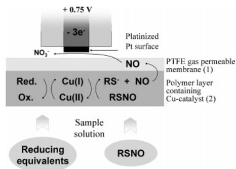
**Figure 1.** Amperometric detection scheme based on catalytic copper species within the outer polymeric layer of proposed RSNO sensor.
