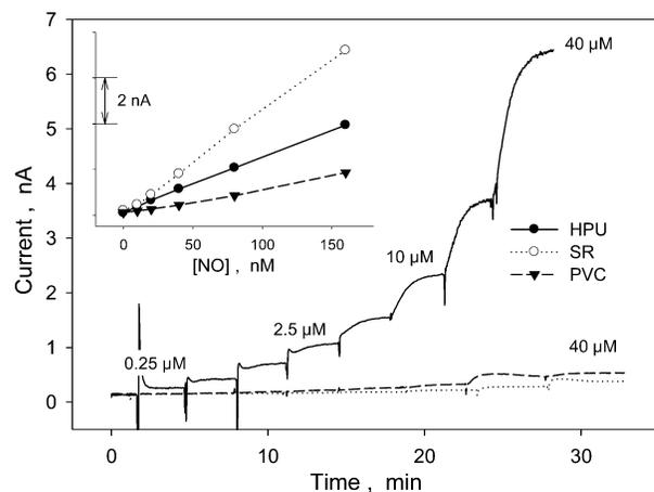
**Figure 2.** Influence of polymer film matrix containing Cu(II)–DTTCT in type I sensors on direct amperometric response toward SNAP and NO (inset). Sample solutions contain 10  $\mu\text{M}$  EDTA and 10  $\mu\text{M}$  ascorbate in pH 7.4 PBS solution.
