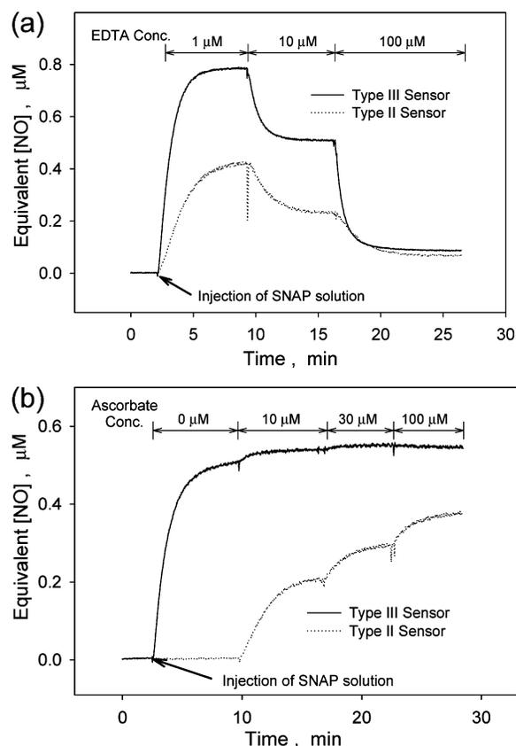
**Figure 6.** Influence of sample phase EDTA concentration (a) and ascorbate level (b) on the amperometric signal of type II and III sensors in response to constant SNAP at 2.0  $\mu\text{M}$ . For (a), ascorbate was present at a constant level of 10  $\mu\text{M}$  in PBS; for (b), EDTA was present at a constant level of 10  $\mu\text{M}$  in PBS.
