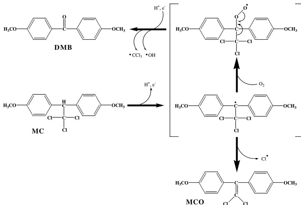
Fig. 1. Possible mechanism for dechlorination of methoxychlor (MC) by MnP-Tween 80 or laccase-HBT treatment. DMB indicates 4,4'-dimethoxybenzophenone; MCO, methoxychlor olefin.
