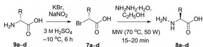
Scheme 2. Preparation of  $\alpha$ -hydrazino acids **8a–8d** (MW = microwave).Table 1. Preparation of  $\alpha$ -bromo acids **7a–7d**.
