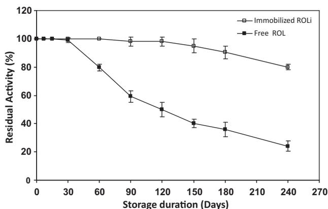
Fig. 6. Residual activity of free and immobilized ROL as affected by incubation at 4 °C after a storage period of 240 days.
