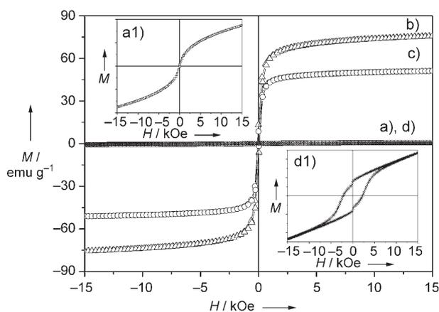
**Figure 4.** Room-temperature hysteresis loops of a) as-synthesized 32-nm truncated octahedral FeO nanoparticles (inset a1: a close look at a section of trace (a)), b) Fe<sub>3</sub>O<sub>4</sub> nanoparticles, c)  $\gamma$ -Fe<sub>2</sub>O<sub>3</sub> nanoparticles, and d)  $\alpha$ -Fe<sub>2</sub>O<sub>3</sub> nanoparticles (inset d1: a close look at a section of trace (d)).
