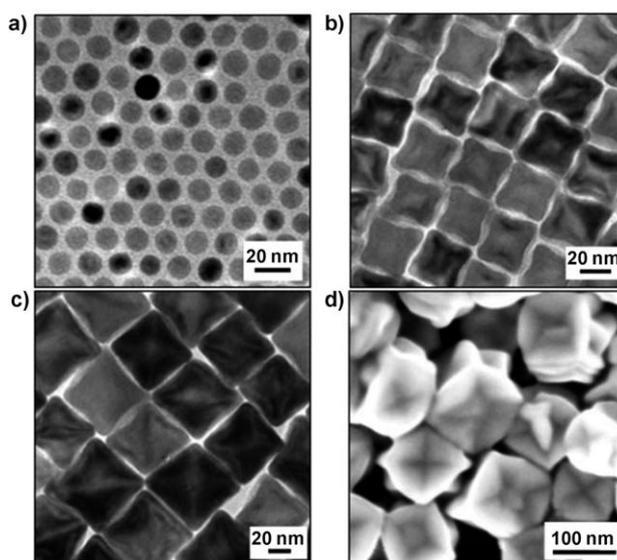
**Figure 1.** TEM images of FeO nanoparticles (the sizes refer to the average lengths of one side in the projected images): a) 14-nm spherical, b) 32-nm, and c) 53-nm truncated octahedral. d) SEM image of 100-nm truncated octahedral nanoparticles.
