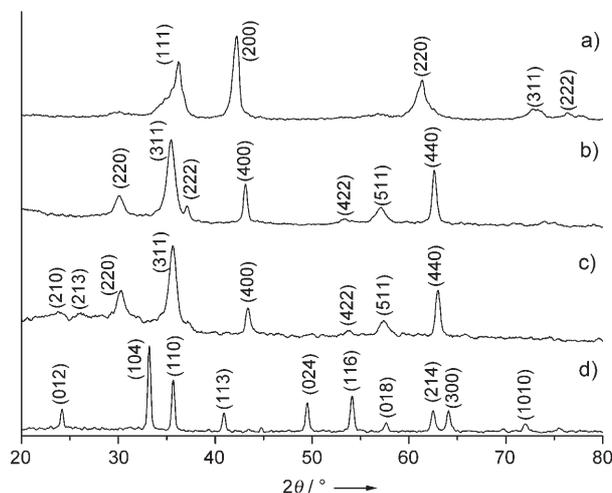
**Figure 3.** XRD patterns of iron oxide nanoparticles: a) FeO, b) Fe<sub>3</sub>O<sub>4</sub>, c) γ-Fe<sub>2</sub>O<sub>3</sub>, and d) α-Fe<sub>2</sub>O<sub>3</sub>.
