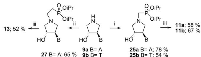
**Scheme 4.** Synthesis of *trans*-nucleotide analogues from pyrrolidine nucleosides. (i) HP(O)(O<sup>*i*</sup>Pr)<sub>2</sub>, formaldehyde; (ii) diisopropyl vinylphosphonate, CH<sub>3</sub>OH; (iii) Me<sub>3</sub>SiBr, DMF (MeCN).
