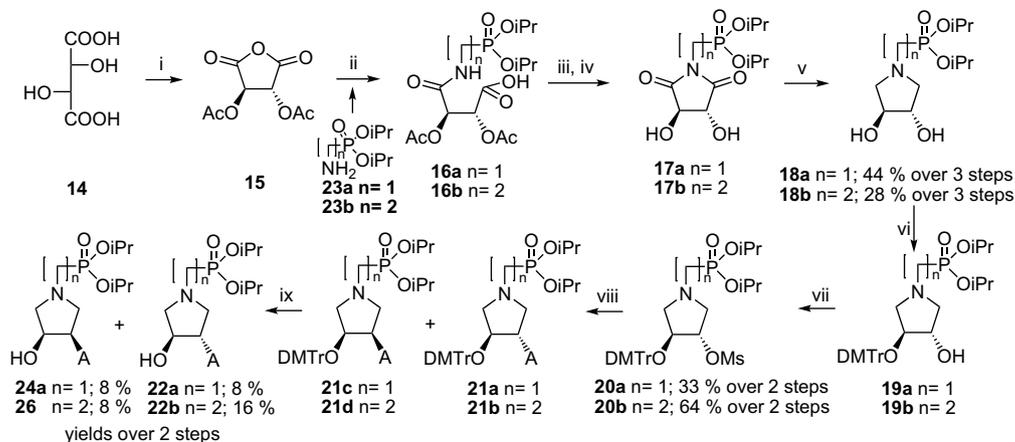
**Scheme 2.** Synthesis of pyrrolidine *N*-alkylphosphonate derivatives. (i) AcCl, reflux; (ii) **23a** or **23b**, DCM; (iii) Ac<sub>2</sub>O, 90 °C; (iv) 1 M HCl in MeOH; (v) NaBH<sub>4</sub>/I<sub>2</sub>/THF, aq HCl; (vi) DMTrCl/pyridine; (vii) MsCl/DMAP/DCM; (viii) Adenine/Cs<sub>2</sub>CO<sub>3</sub>/DMF; (ix) 80% aq AcOH.
