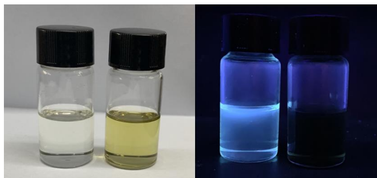
FIGURE 3 Comparison of the probe H 2 L and L-Cu 2+ solution under normal light (left), and comparison between H 2 L and L-Cu 2+ solution under 365nm UV lamp (right).
