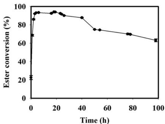
Figure 4. The continuous synthesis of dodecyl oleate in a packed bed reactor. The synthesis was catalyzed by bagasse from petioles using isoctane as the reaction solvent and a 0.2 M final substrate concentration (molar ratio 1:1) at 50 °C.
