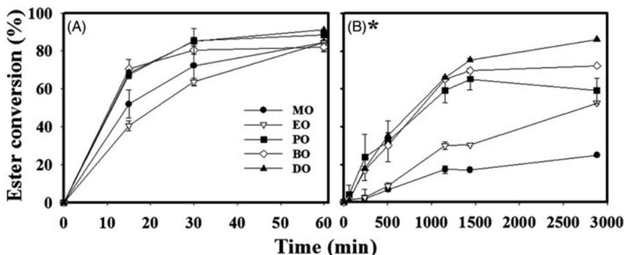
Figure 2. Kinetics for the synthesis of oleic acid esters. (A) Treated lyophilized latex, *TLL*; (B) bagasse from petioles, *BP*. Synthesis was performed at 50 °C using isoctane as the reaction solvent. \*37.5 mg BP/mL. MO – methyl oleate; EO – ethyl oleate; PO – propyl oleate; BO – butyl oleate; DO – dodecyl oleate.
