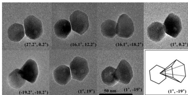
**Figure 3.** TEM images of hexagonal pyramid shaped ZnO nanocrystals at various tilted angles ( $X^\circ$ ,  $Y^\circ$ ) (left: hexagon shape, right: from hexagon shape to hexagonal pyramid image).
