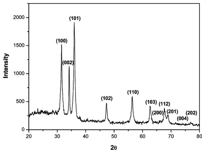
**Figure 1.** XRD pattern of hexagonal pyramid-shaped ZnO nanocrystals.
