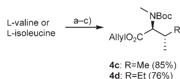
Scheme 6. Syntheses of NMeVal and NMeIle units. a) Boc 2 O, Na 2 CO 3 , H 2 O, RT; b) NaH, MeI, THF, 0 °C → RT; c) allyl bromide, K 2 CO 3 , DMSO, RT.
