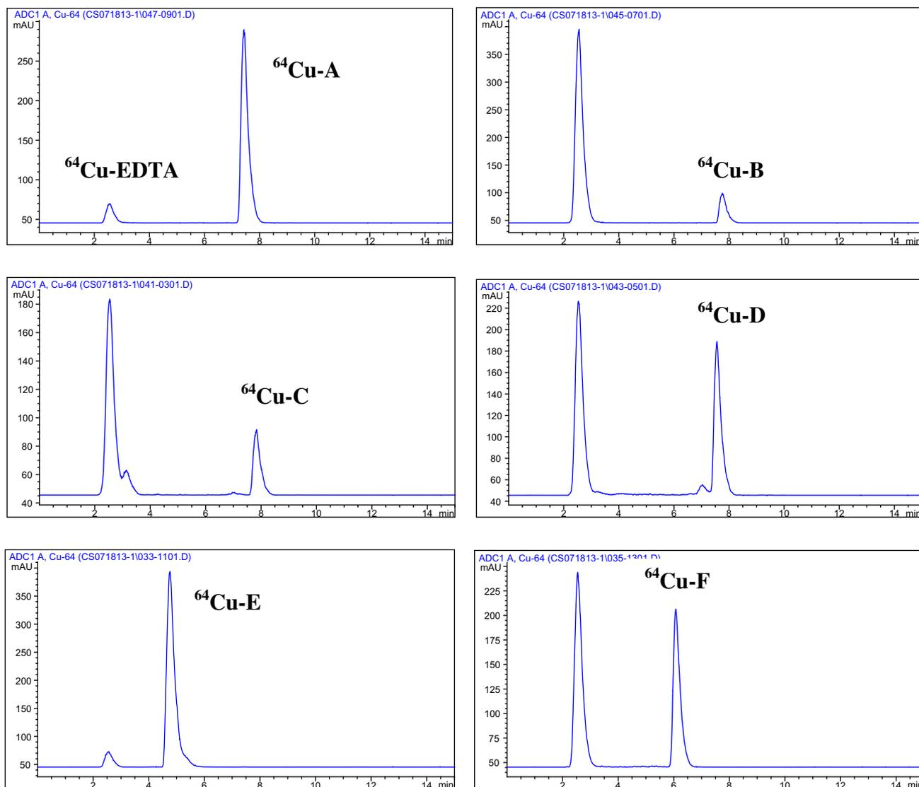
Figure 3. HPLC chromatograms of  $^{64}\text{Cu}$ -radiolabeled complex against EDTA challenged for 25 h (37 °C, pH 5.5).
