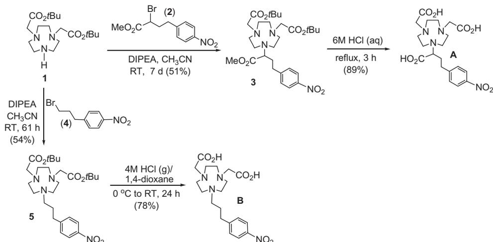
**Scheme 1.** Synthesis of TACN-based chelators A and B.
