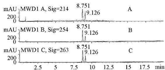
Figure 2. The HPLC chromatogram of the crude reaction mixture resulting after the coupling between 3 and 4, in dichloromethane and using pyridine as base, at  $\lambda = 214$  (A), 254 (B) and 263 nm (C), respectively
